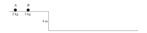
Two small spheres A and B of masses 2 kg and 3 kg respectively lie at rest on a smooth horizontal platform which is fixed at a height of 4 m above horizontal ground (see diagram). Sphere A is given an impulse of 6 N s towards B, and A then strikes B directly. The coefficient of restitution between A and B is  $\frac{2}{3}$ .
